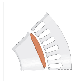
Sectional drawing DC motor with surface magnets (bread loaf)
