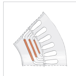
Sectional drawing FS motor with interior permanent magnets and reluctance torque use
